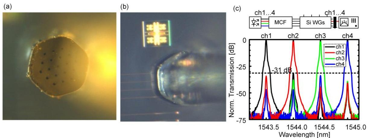
**Fig. 1** Multicore fiber: (a) facet with 19 channels; (b) top view when coupling to four channels on chip. (c) Optical interchannel crosstalk below -31 dB for four channels. The spectra were obtained by coupling four different wavelengths to the multicore fiber.
